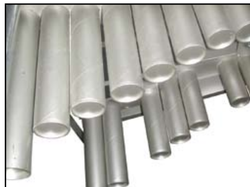
Close-up view of the cardboard resonators, showing the capped ends and mounting box.
