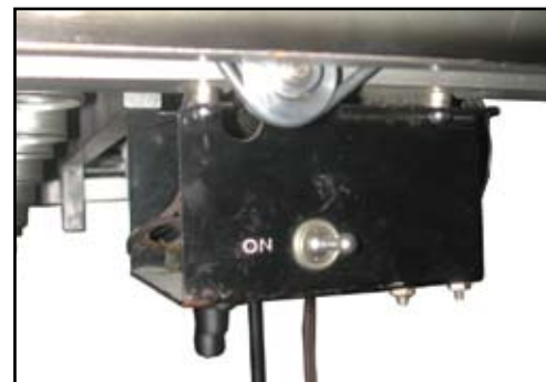
Close-up of motor for the rotating fans. Note the simple "on/off" toggle switch and one-speed pulley.
