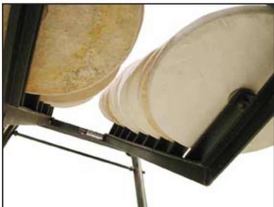
View from below, showing the mounting system for each disk.
