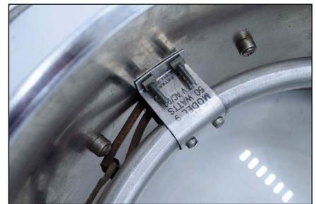
Internal mounting bracket for Damp-Chaser Model 9 dehumidifier.
