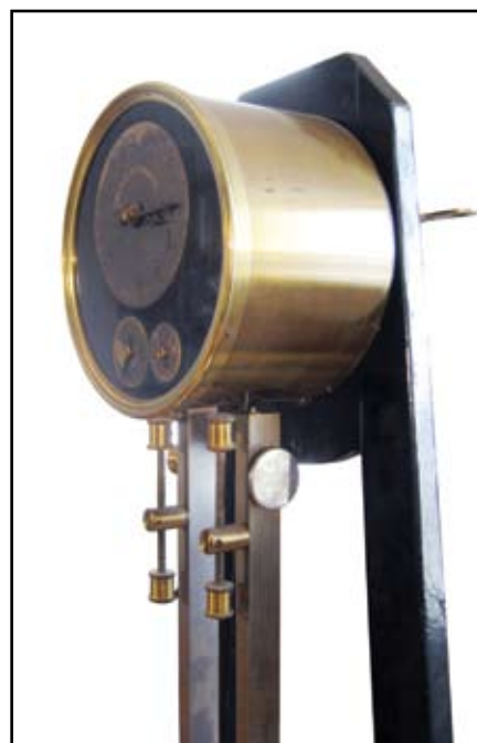
Detail showing the dials for hours, minutes and seconds and the threaded brass weights, which adjust the speed of vibration of the fork
