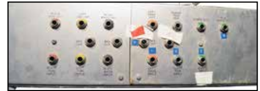
Back of Percussion Coupler showing input and output connections)
