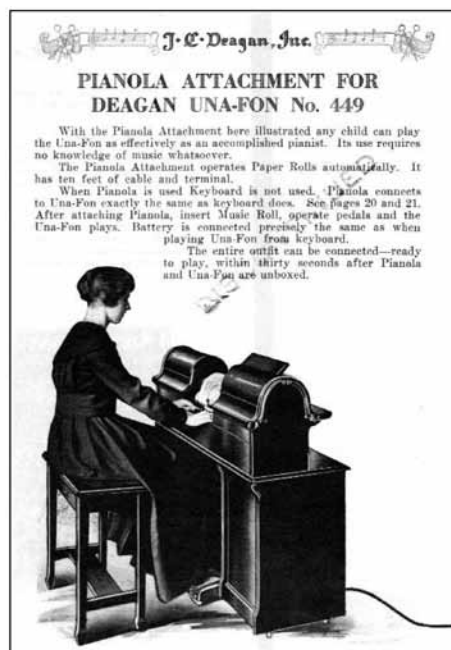
Figure 7. Deagan automated the Unafon by adding a piano roll playing unit. Electrical contacts were added to the device to make it functional.
