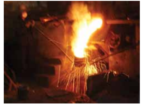
Molten metal is poured into a raw disk shape.
