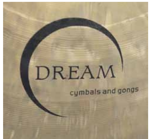
Detail of gong showing the company logo. Note the circular lathe marks, as well as the radial hammered lines.
