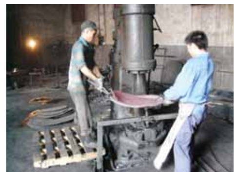
Initial machine-hammering of a gong at the factory.
