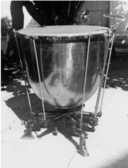
Charles White's Schnellar drum (in his backyard) with added counterhoop. Notice the electrical plug at the bottom for a heating device installed for natural skin heads.
