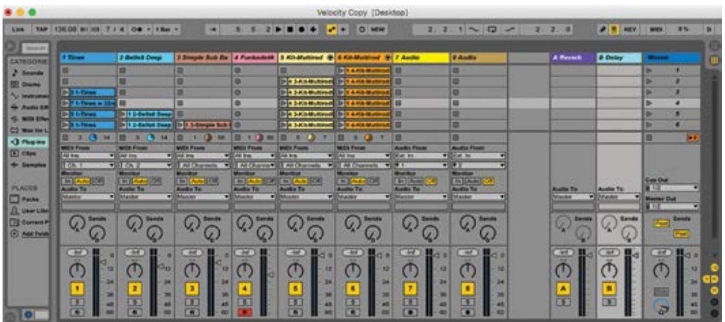
Live’s session view, in which audio and/or MIDI clips (individual cells) are organized in scenes. Typically, each column contains like MIDI or audio clips. Each row represents the clips that comprise each scene. Launching a scene activates all of its clips simultaneously.
