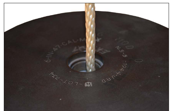
Rear (top) end of the shell, showing stamped manufacturing information. Note the rope inserted into the threaded primer hole.
