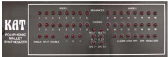
Detail of the control panel showing the instrument name and multi-bank sequencer for two voices.
