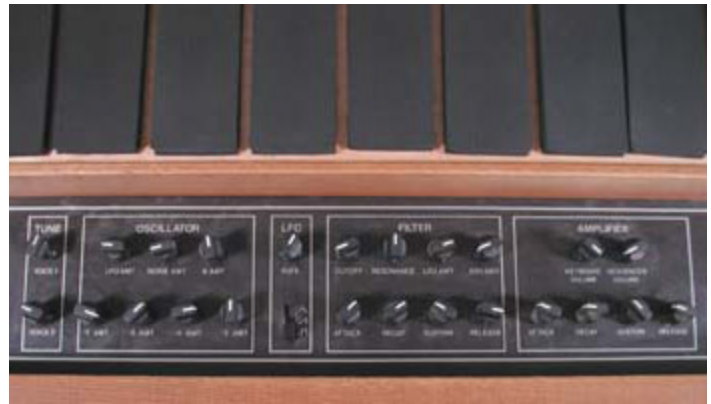
Detail of the control panel showing knobs for tuning, oscillator, LFO, filter, and amplifier
