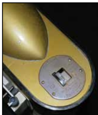
Electronic Marimba Metronome (arrow up = Largo, arrow down = Presto)
