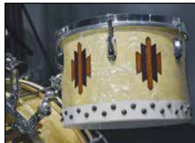
Closeup view of a tom-tom showing tacked head, decorated finish, and Zephyr lugs with claw hooks.
