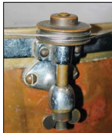
Close-up of a tuning lug with Anheier spool and cable
