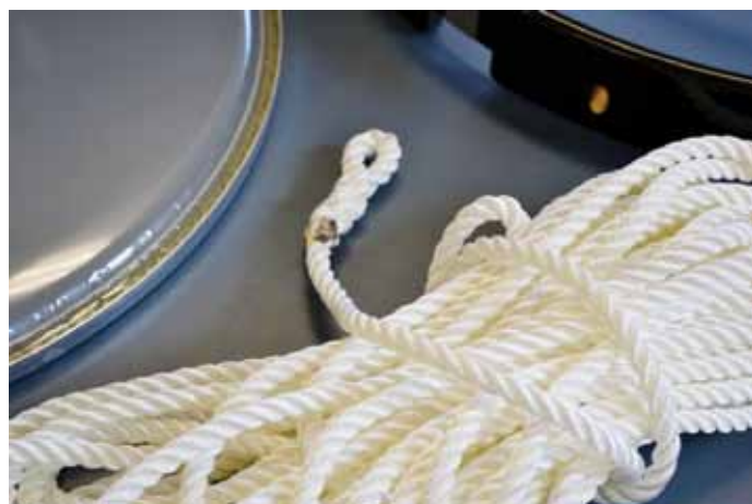
Dacron rope that is laced around the drum as a tension system. Shown is the eyelet braided on one end, through which the pigtail is tied.
