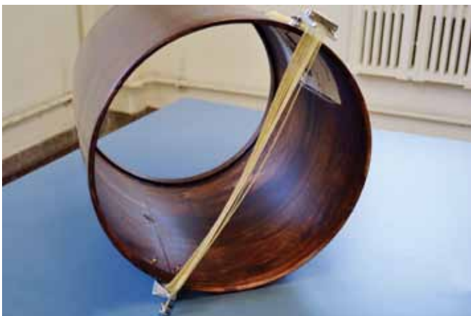
Inside view of the 17" x 18" snare drum. Note the interior seam of the single-ply steam bent maple shell.
