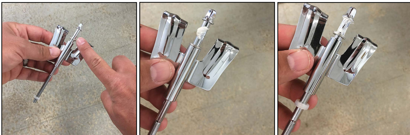
Example 5: Applying lithium grease to the top of the lug
