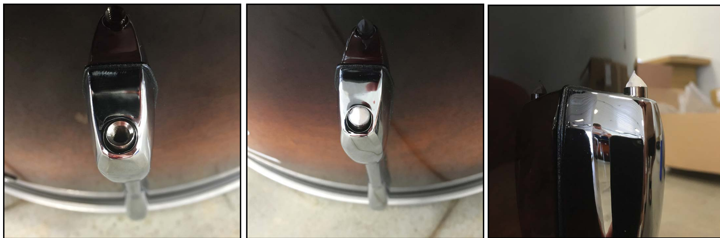
Example 6: Apply lithium grease to the top of the lug
