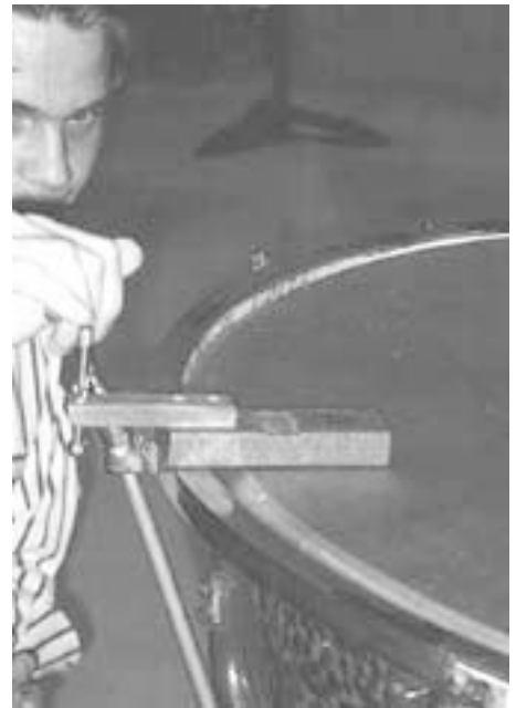
Using the altered Mark Yancich Tap Device to create an even collar. Note that the head is tucked German style and that I am using the flat part of the wood in this case instead of the screw tip on the counterhoop.
