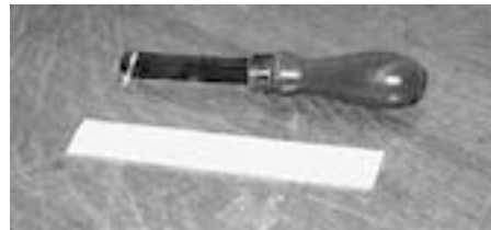
Head Tucking Tool. It is about six inches long. The wooden handle is attached to a thin piece of brass with an upturned end to make it easier to push the head under the flesh hoop.
