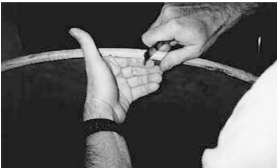
Photo 5. I smooth the head on the hoop after it is tucked to eliminate any bunching up of the material. I wet the tucking tool as I perform this operation so as to avoid cutting the head accidentally.
