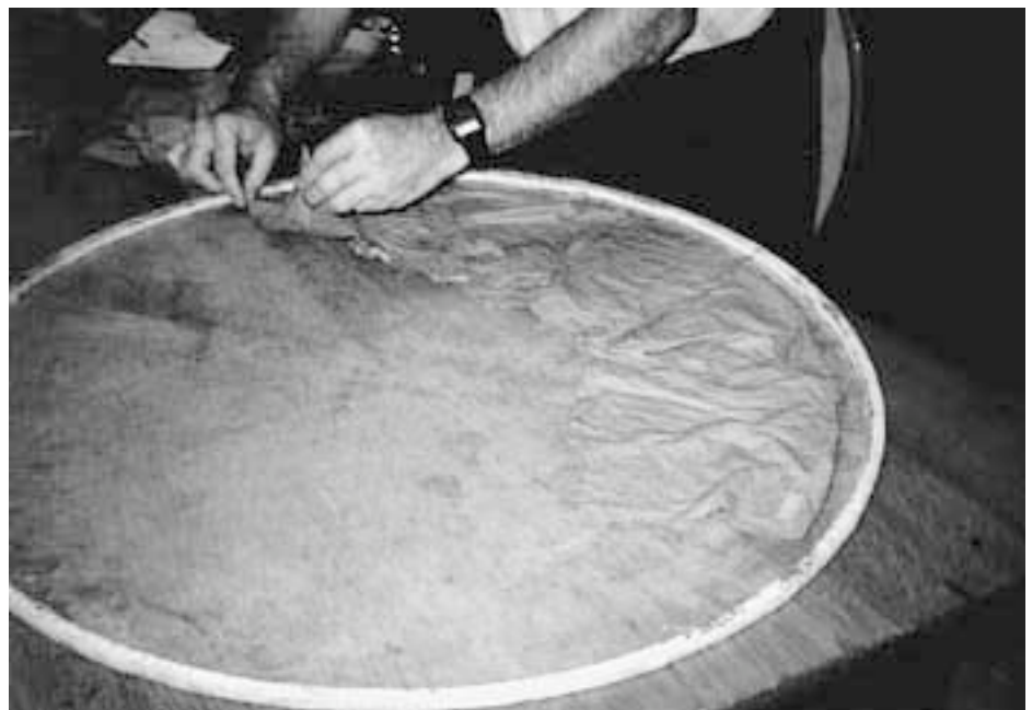
Photo 6. I place damp paper towels on the head to within one inch of the hoop so that the head dries slowly.
