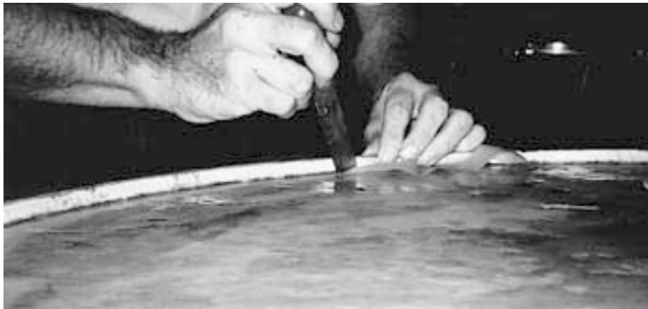
Photo 4. The tucking process consists of carefully pushing the head under the hoop as the hoop is lifted slightly. Note how I hold the material up against the hoop with my left hand as I push it under with the tucking tool in my right.
