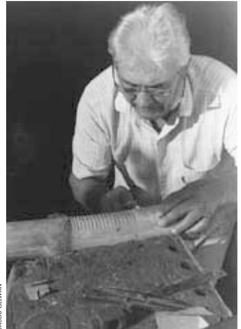
Photo 1. Luthier Nadir Rovari building a bamboo reco-reco , with a small saw and knife.
