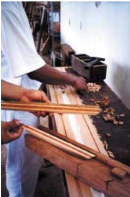
A decorative "signature" front piece is being assembled.
