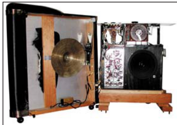
The interior of the prototype instrument is installed on a "two-by-four" wooden frame.
